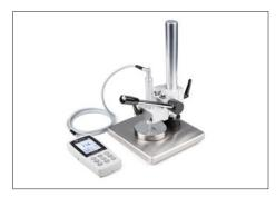
Test stand for repeatable movements during testing. In this way you can avoid errors which could occur in manual handling of the sensor.
