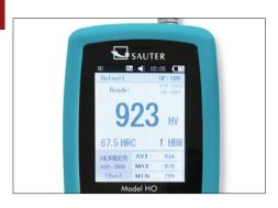
Mini statistics function: Display of the measuring result, the number of measurements, the maximum and minimum value as well as the average value and the standard deviation
