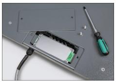
Easy levelling of the weighing bridge as well as access to the junction box from above
